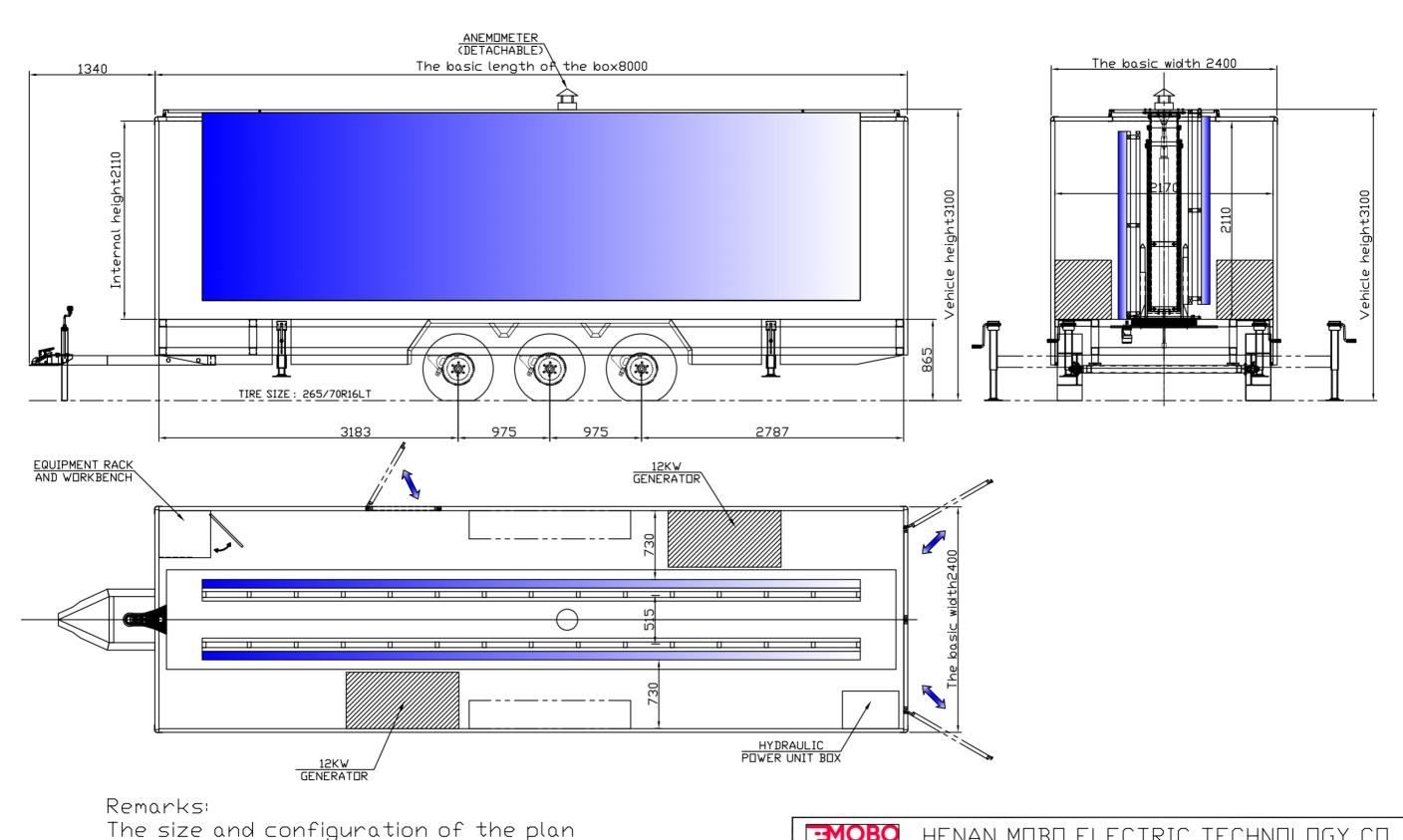
The size and configuration of the plan are for reference only. The actual contract and design requirements are the basis for the specific production.
